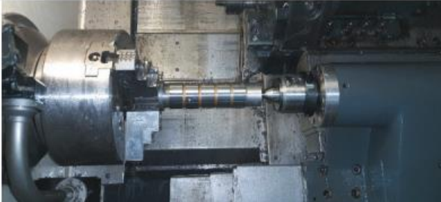
Fig. 2. Turning the samples on the CTX 310 ECO lathe
