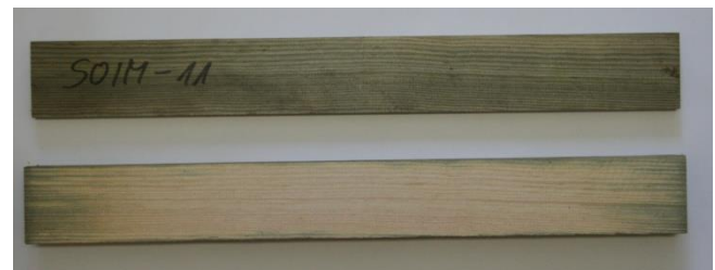
Fig. 1. Sample of impregnated pine wood (SOIM-11 sample number). An external surface is shown at the top, and the inner surface after cutting is shown below
