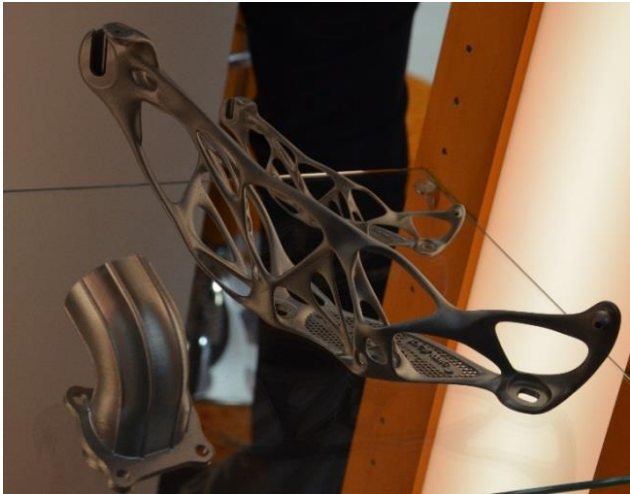
Fig. 2. Automotive components manufactured using DLMS/SLM topology optimization
