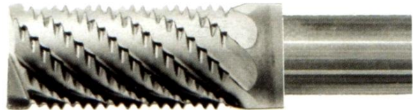
Fig. 13. End mill with diamond coating with stepped edges, for processing composite materials (Prototype-Werke)
