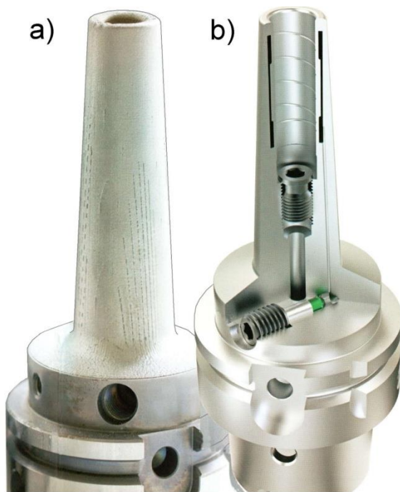
Fig. 24. Examples of bodies of hydraulic holders printed with 3D technique: a) printed part to the grip part, b) section of the frame after execution (MAPAL)
