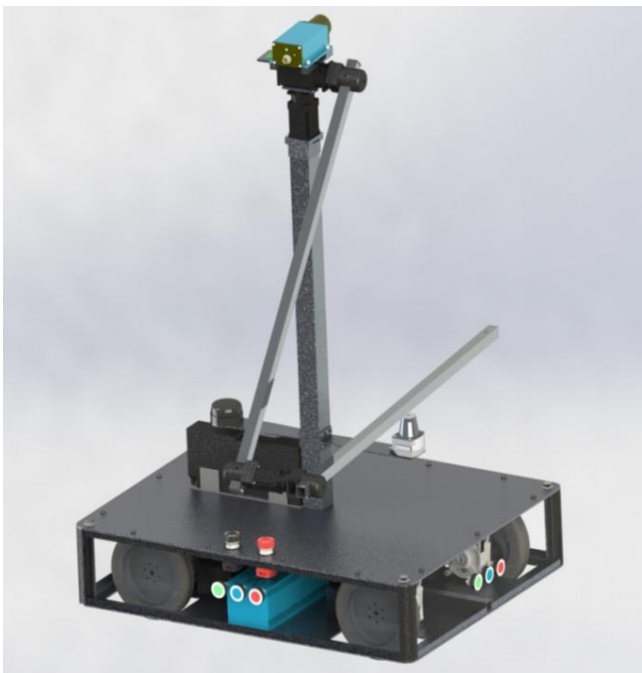
Fig. 4. Visualization of the model of the system supporting the measurement of noise emissions
