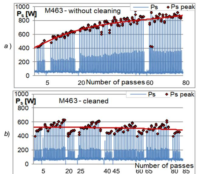
Fig. 4. Grinding power of the AZ31HP alloy grinding wheel with a grinding wheel: a) traditionally loaded, b) assisted cleaning
