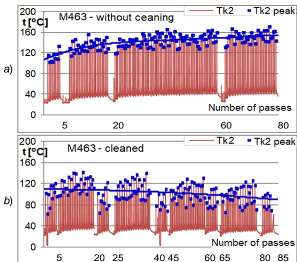
Fig. 5. Temperature of grinding the K-type thermocouple placed in the AZ31HP alloy sample with a grinding wheel: a) traditionally pulled, b) assisted cleaning
