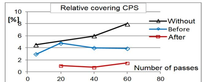
Fig. 3. Characteristics of wheel grinding changes in two ways of the process: traditional (without cleaning) and assisted cleaning (before cleaning, after cleaning)
