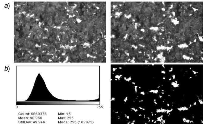
Fig. 2. Development of GWCS plug-in during AZ31HP grinding (a), brightness histogram and binary GWCS image (b)
