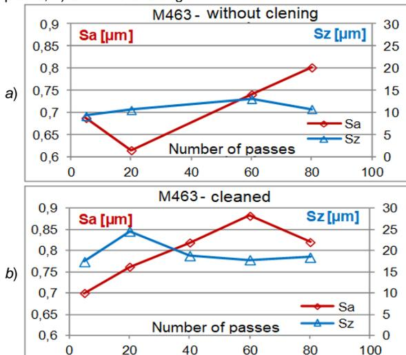
Fig. 6. Surface geometrical structure of AZ31HP alloy specimen ground with grinding wheel traditionally (a) and assisted with cleaning (b)
