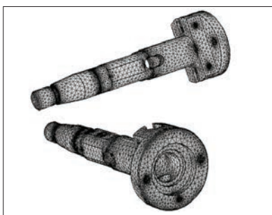
Fig. 2. FEM mesh model used in the designed shaft
