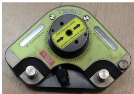
Fig. 5. FIXTUR LASER T220 laser head with transmitter [6] Rys. 5. Głowica laserowa FIXTUR LASER T220 z nadajnikiem [6]
