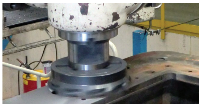
Fig. 3. Two-angle head with mounted sanding head \varnothing 160 by Sandvik during machining [6]
