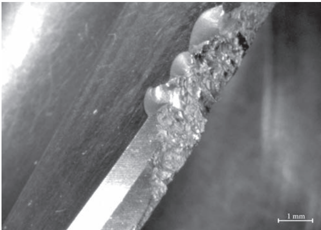
Fig. 3. Application surface after machining time t_s = 44 min 11 s in variant 1 ( VB_B = 1,362 mm)
