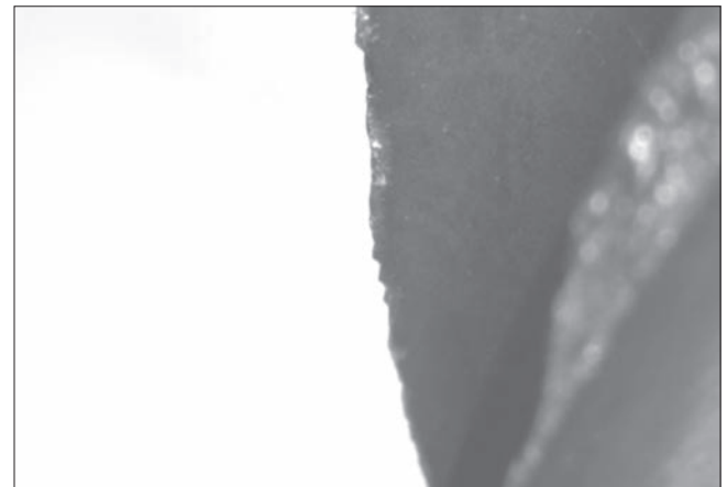
Fig. 7. Rake surface after machining time t_s = 44 min 11 s (variant 1)
