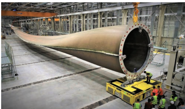
Fig. 1. The effect of the process of forming a 107 m 12 MW wind turbine blade, LM factory in Cherbourg, France, project manager MSC. Łukasz Cejrowski (graduate of WIM UTP, Bydgoszcz) [21]
