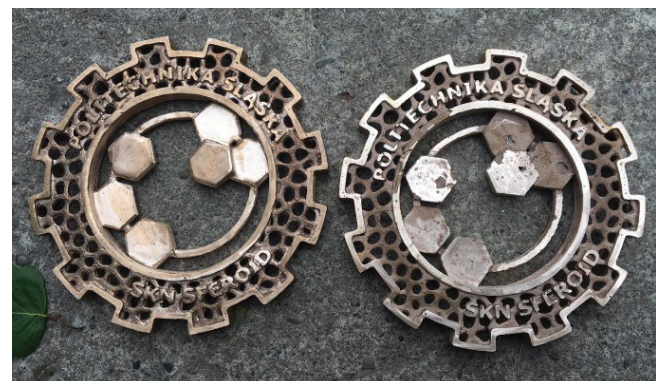
Fig. 6. Comparison of the results: a) casting made with risers in the middle of the model, b) casting with the risers used only on the edges
