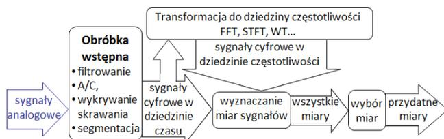
Fig. 2. General scheme of signal processing in DNIPS
