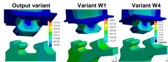
Fig. 3. Equivalent (von Mises) stress distribution, MPa
