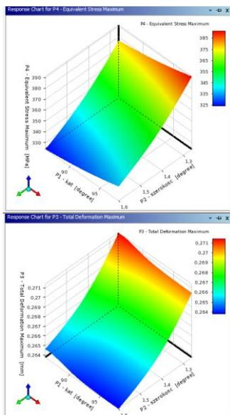
Fig. 2. Influence of parameters P1 and P2 on the distribution of equivalent (von Mises) stress and deformations at rotational speed  $\omega = 927$  rad/s
