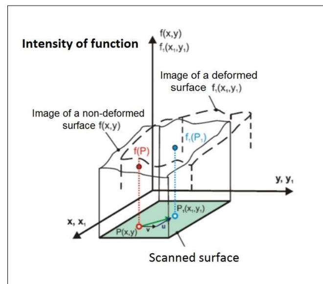
Fig. 5. Analysis scheme of undeformed and deformed surface image [1]
