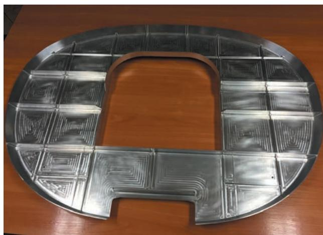
Fig. 2. Ready-made frame of an airplane produced in the milling process
