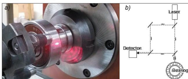
Figure 5. Contactless measurement of vibration speed with a laser vibrometer, the beam of which is visible on the outer ring of the rolling bearing (a), and the principle of measurement (b)
