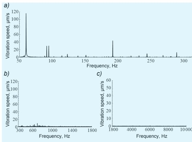
Fig. 2. Spectrum of velocity of rolling bearing type 6204 - electrodynamic sensor measurement SG 4.3: a) low frequency band, b) medium frequency band, c) high frequency band
