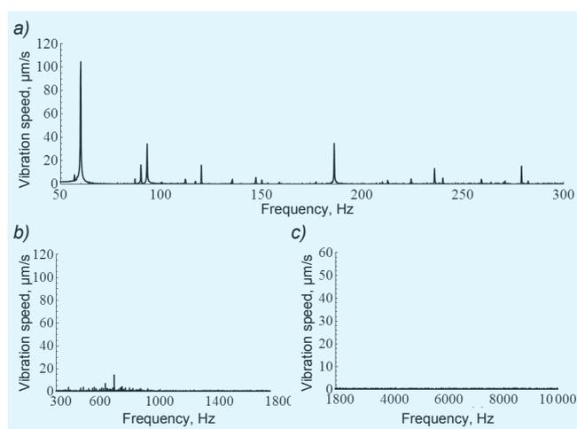
Fig. 6. Spectrum of velocity of rolling bearing type 6204 - measurement by PSV-500 laser vibrometer: a) low frequency band, b) medium frequency band, c) high frequency band
