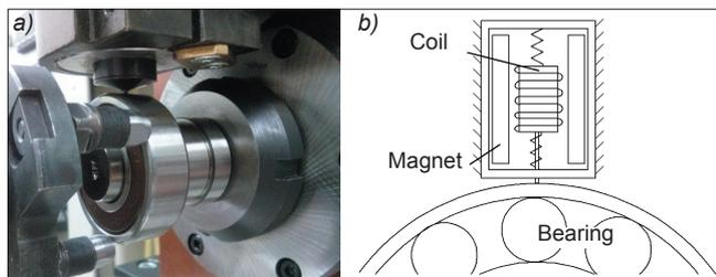
Fig. 1. STPPD accelerometer equipped with an electrodynamic sensor (a) and a diagram of the relative velocity measurement (b)
