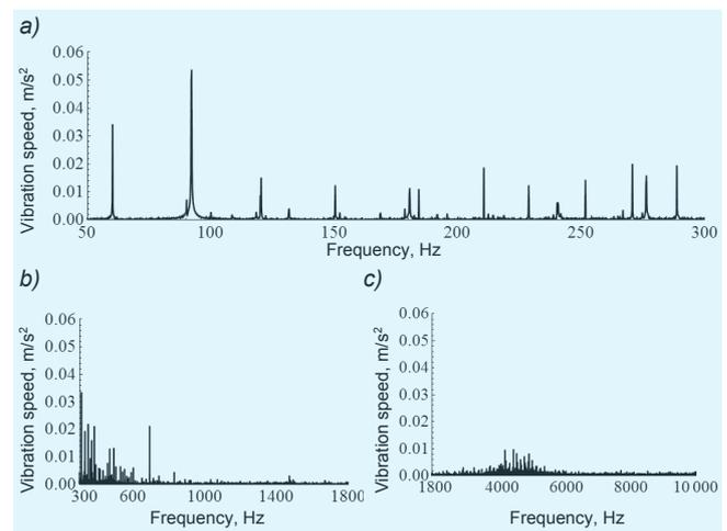
Fig. 4. Spectrum of the vibration speed of a type 6204 rolling bearing mounted in a housing - piezoelectric sensor measurement 608A11: a) low frequency band, b) medium frequency band, c) high frequency band
