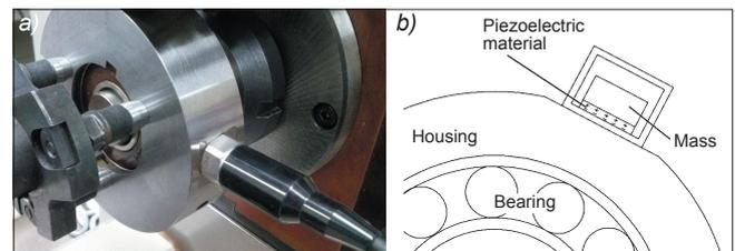
Fig. 3. STPPD measuring station equipped with piezoelectric accelerometer (a) and the scheme of absolute vibration acceleration measurement (b)
