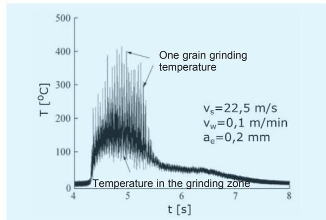
Fig. 8. Example of recorded temperature signal during grinding with discrete grinding feed with cBN abrasive [4]
