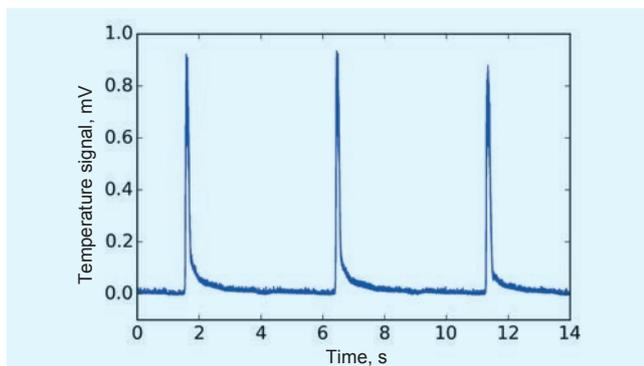
Fig. 6. Example of a recorded natural thermocouple signal for the subsequent three grinding wheels
