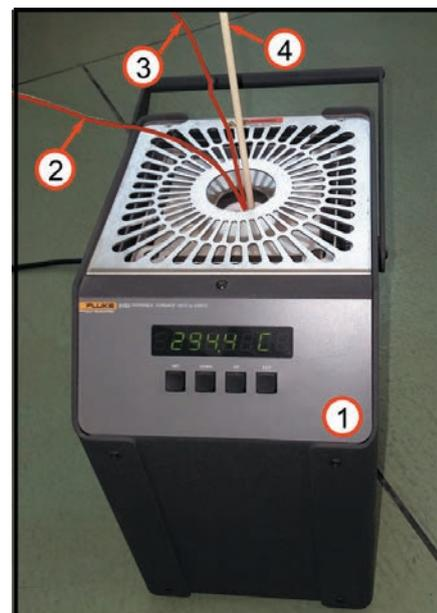
Fig. 1. The thermocouple calibration furnace (1) with the calibrated thermocouple (lines 2 and 3) and the reference thermocouple (4)
