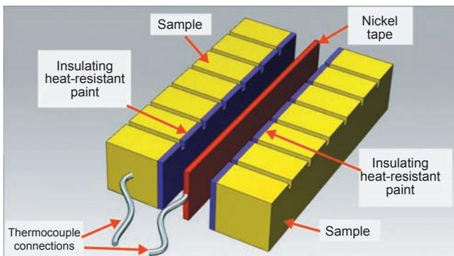
Fig. 5. Diagram of the construction of the natural thermocouple used in the tests
