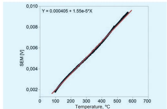
Fig. 4. Regression line describing the characteristics of the thermocouple
