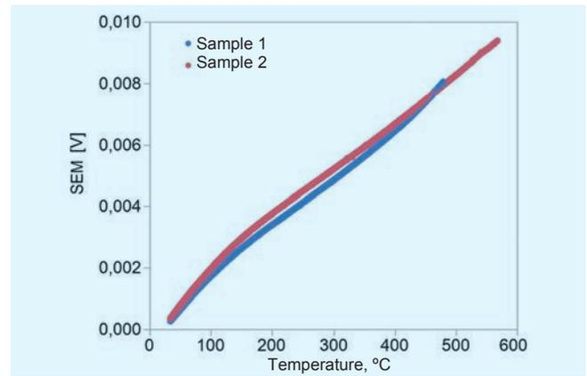
Fig. 3. SEM electromotive force values according to temperature in two samples representing natural thermocouple
