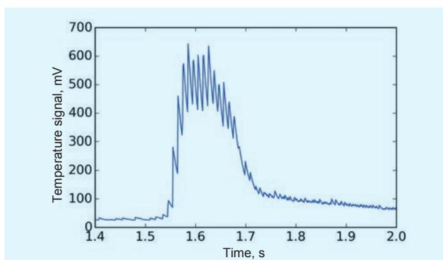
Fig. 7. Temperature values during a single grinding wheel passage
