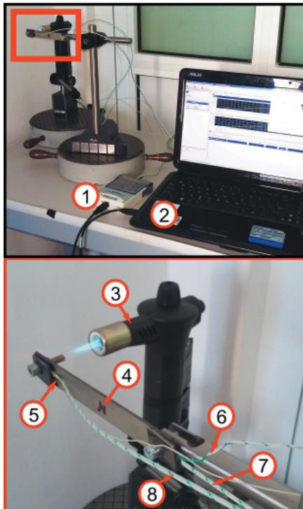
Fig. 2. Stand for calibrating the thermocouple (1), PC (2), gas burner (3), steel thermocouple element (4), nickel thermocouple element (5) (6), thermocouple measuring the temperature of the cold end of the steel element (7), reference thermocouple relative to the calibrated one (8)
