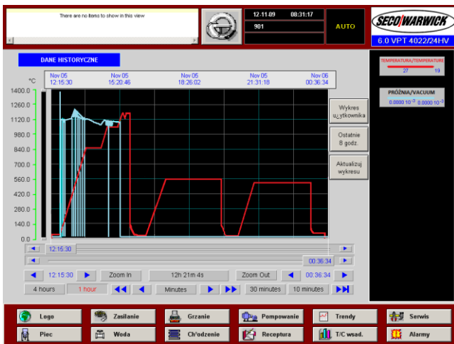
Fig. 1. Course of heat treatment of high speed steel plates in SECO/WARWICK vacuum oven type 6.0VPT-4022/24IHV: red line – temperature; aquamarine line – pressure
