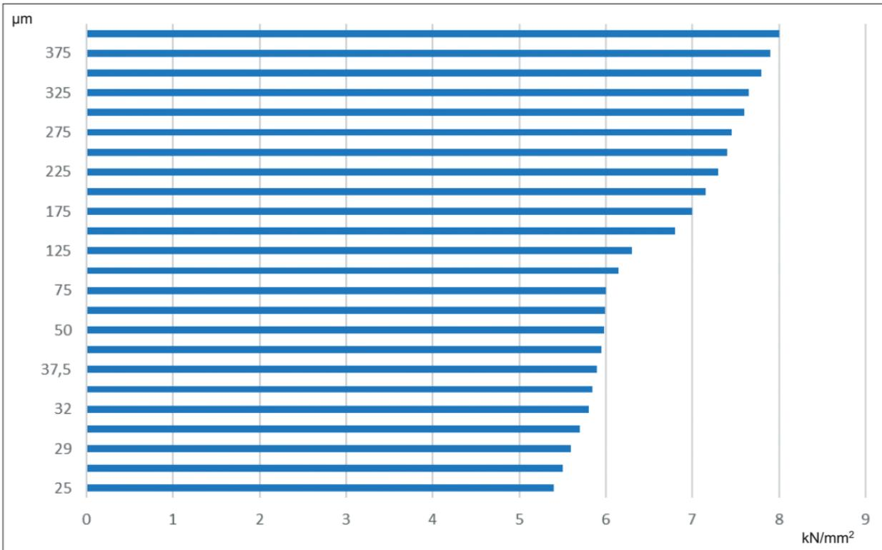
Fig. 8. Values of meso-hardness (determined by Knoop's method) and its depth in TWW gear teeth after grinding
