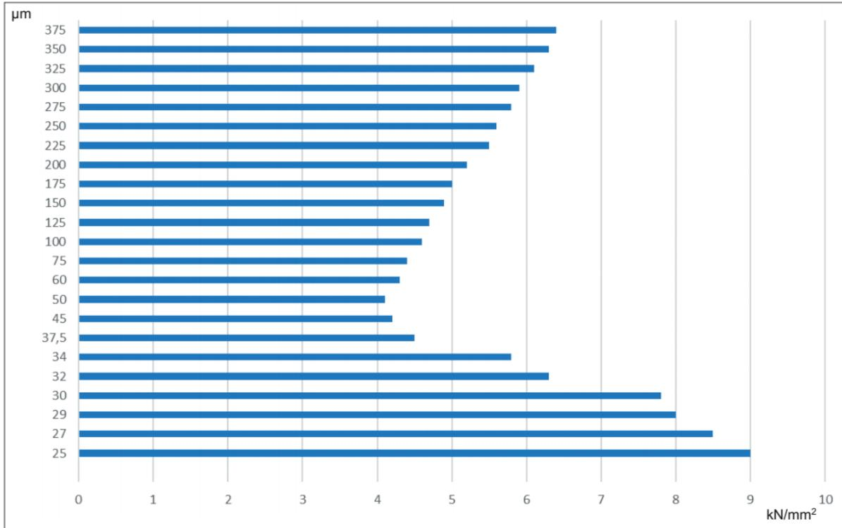
Fig. 7. Distribution of meso-hardness (determined by Knoop's method) in TWW gear teeth after grinding
