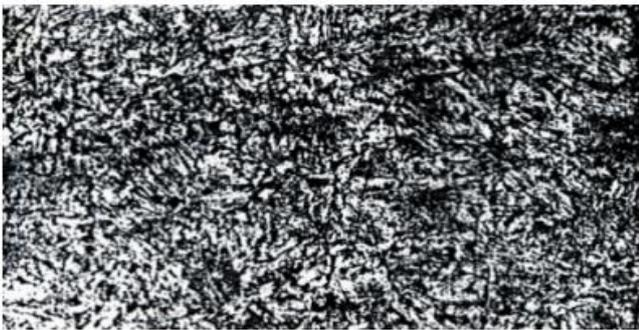
Fig. 2. Microstructure of gear tooth of 12H2N4A steel ( $\times 500$ )
