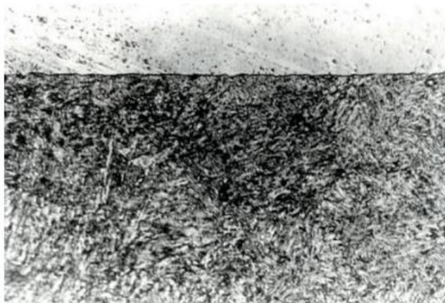
Fig. 3. Microstructure after grinding of 40H steel gear ( $\times 500$ )
