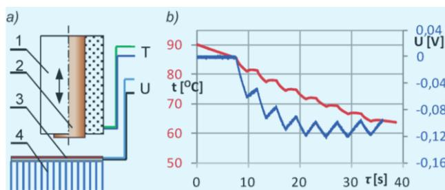
Fig. 2. Peltier module calibration system (1 – thermal insulation, 2 – copper rod, 3 – Peltier module, 4 – heat sink) (a); change of the Peltier's thermoelectric voltage and the temperature of the balance system (b)
