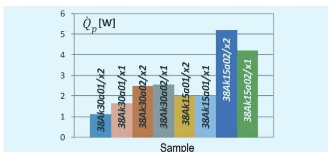
Fig. 5. Absolute value of the heat flux transmitted to the Peltier module
