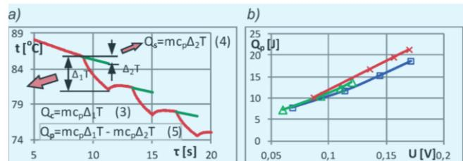
Fig. 3. Temperature diagram of the balance system during 3 control contacts (a); characteristics of the Peltier module: thermoelectric voltage – heat (b)
