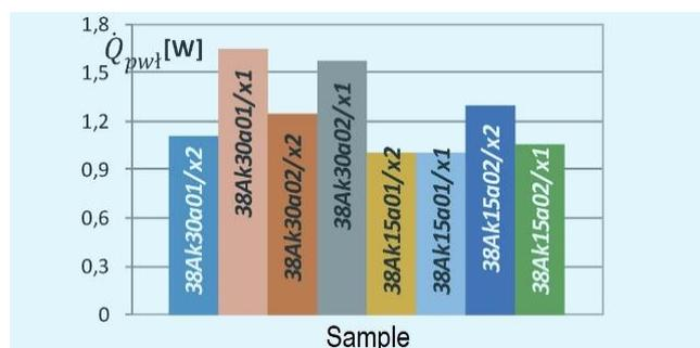
Fig. 6. Heat flow transmitted to the Peltier module relative to the amount of wheel material carried by the stream
