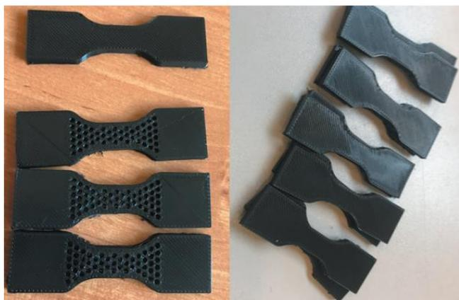
Fig. 7. Samples prepared for testing
