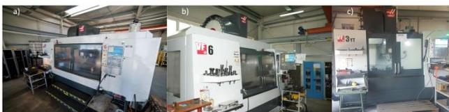
Fig. 2. Tested milling centers: a) VF-7/50, b) VF-6/50, c) VF-3YT/50
