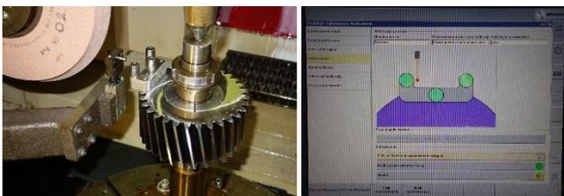
Fig. 4. Calibration of the lower external measuring arm on the Rapid Höfler 900 grinder
