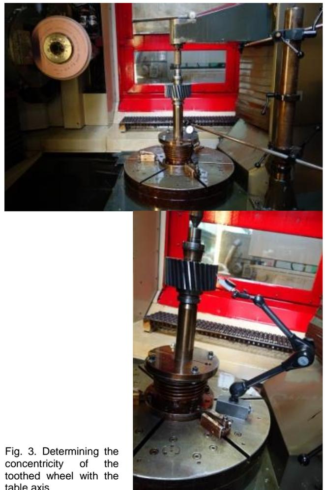
Fig. 3. Determining the concentricity of the toothed wheel with the table axis
