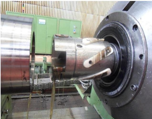
Fig. 2. Tool for drilling holes in risers
