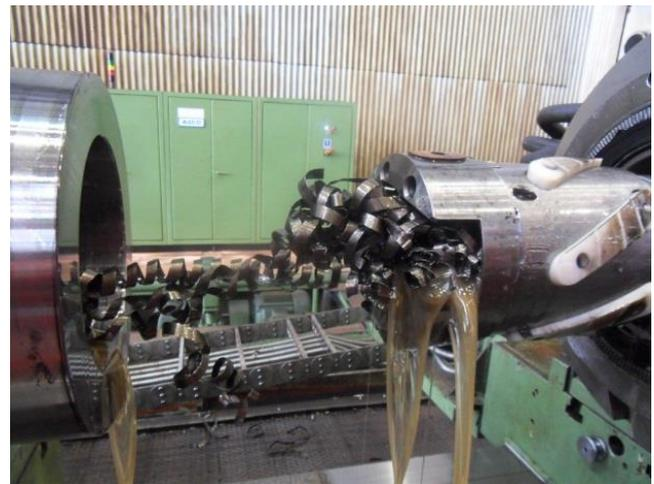
Fig. 4. Form of chips making their removal difficult
