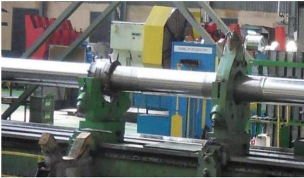
Fig. 1. Method of supporting the riser during the turning process
