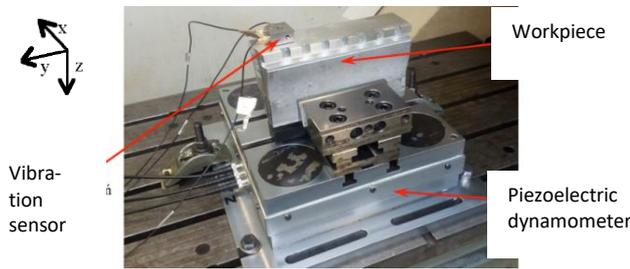
Fig. 1. Way of fixing the workpiece
