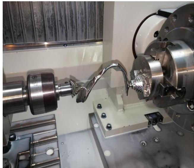
Fig. 3. Machining system with the device and object (finishing)
