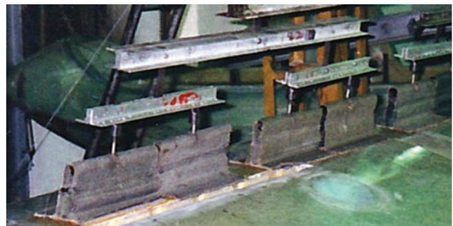
Fig. 13. Patches bonded to the wing's surface (author: Wojciech Frączek)
