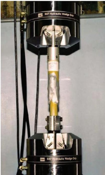
Fig. 2. Model tests of a composite joint connecting duralumin pipes
