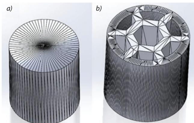
Fig. 2. Samples in stereolithography language (.stl): a) MED 610 sample without cell structure; b) sample with cell structure
