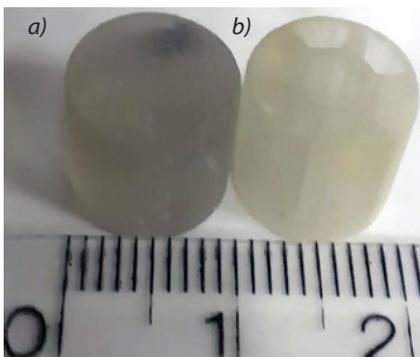
Fig. 3. Samples printed from MED 610: a) MED 610 sample without cell structure; b) sample with cell structure
