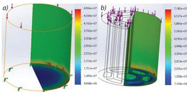
Fig. 8. Samples in Solidworks Simulation: a) sample MED 610 without cell structure; b) sample with cell structure
