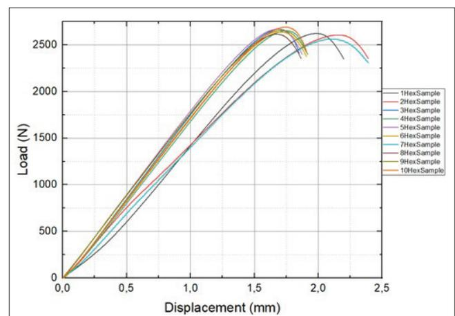
Fig. 6. Plot Load – displacement for 10 samples with hexagonal cell structure
