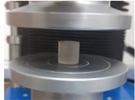
Fig. 5. The specimen placed between the plates prior the compression test
