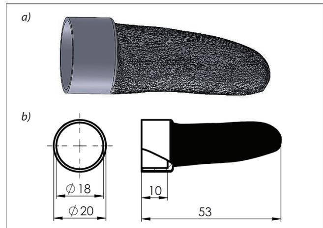
Fig. 7. Rebuilt model of the little finger: a) Solidworks part, b) little finger dimensions
