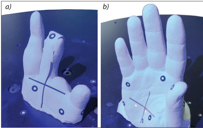
Fig. 4. Scanning the model of: a) damaged left hand and b) right hand
