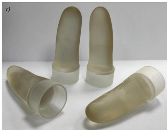
Fig. 9. Printout: a) before removing support material, b) cleaned fingers, c) cleaned fingers with sleeve
