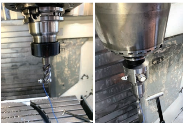
Fig. 3. Stand for testing the stability of the milling process: tools with a vibration sensor mounted on the machine tool
