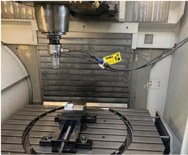
Fig. 7. Stability of the milling process during HSC machining of an aircraft structure element
