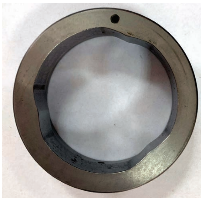
Fig. 3. Injection pump cam ring subjected to manganese phosphating (slip)
