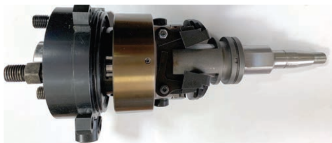
Fig. 2. Pump assembly with components subject to high wear
