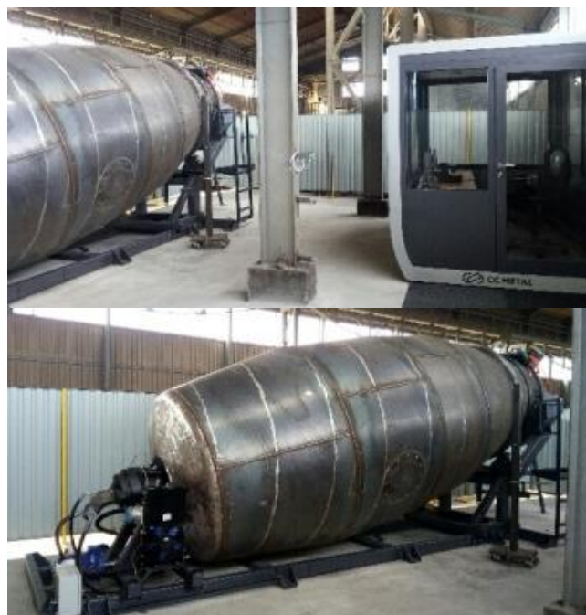
Fig. 2. Test stand – test object – 12 \text{ m}^3 mixer
