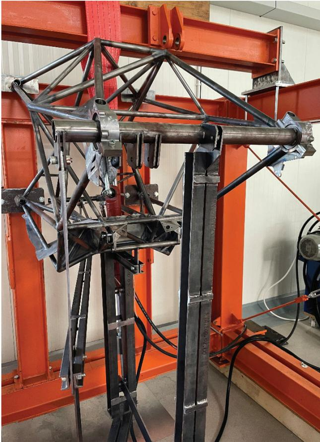
Fig. 3. Engine bed truss mounted on static test stand with marked measurement points
