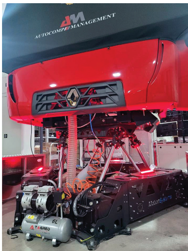
Fig. 2. Firefighting vehicle simulator mounted on a six-degree-of-freedom motion platform
