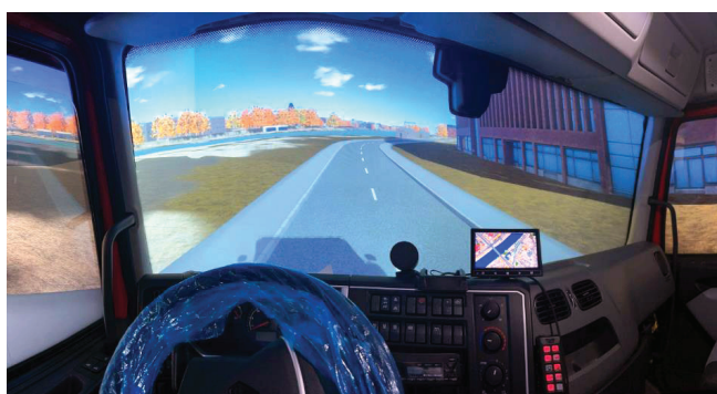
Fig. 6. Firefighting vehicle simulator – In-Cabin Visual Projection Geometry Setup
