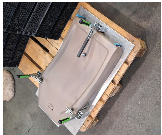
Fig. 2 Method of mounting the molding on the fixture and orientation of the X/Y axes relative to the melt flow direction (source: own work)
