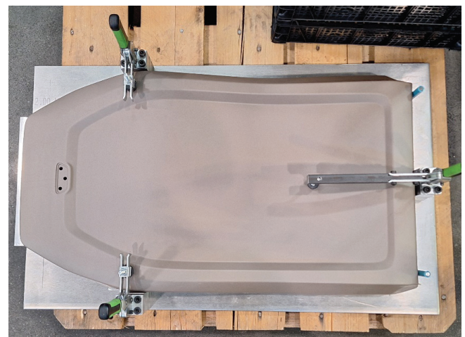
Fig. 3 Support and locking points for the part width along the Y-axis (source: own work)
