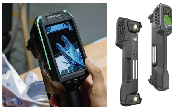
Fig. 5. Creaform HandySCAN EVO laser scanner (left) and HandySCAN EVO MAX laser scanner (two images on the right), featuring a display integrated into the scanner head Rys. 5. Skanery laserowe HandySCAN EVO (po lewej) i HandySCAN EVO MAX (dwa obrazy po prawej) firmy Creaform z wyświetlaczem w głowicy
